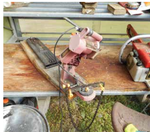
A cheap chain grinder from Harbor Freight makes up for poor filing.
